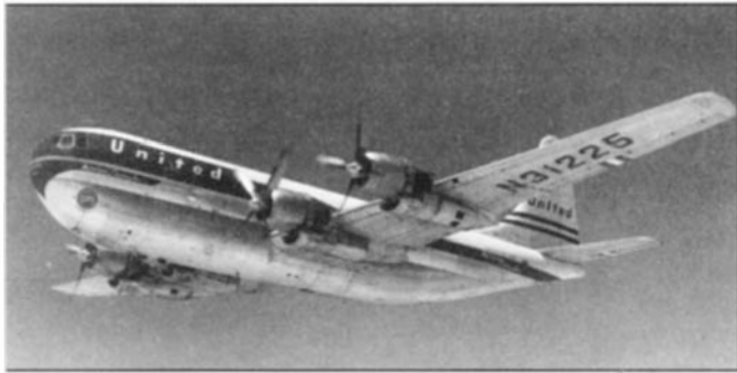
A Boeing 377 Stratocruiser in flight. These double-deck planes, built to carry over 100 passengers, went into service between the West Coast and Hawaii in 1950.
