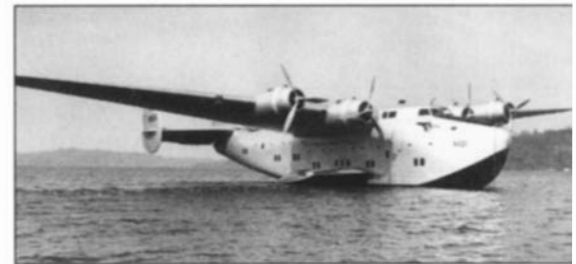
The Boeing 314 flying boat, put into service by Pan American in 1939. The flying boat had a range of 3,500 miles and could attain a speed of 193 miles per hour.
